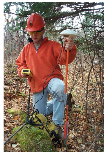
Field crews use Global Positioning System (GPS) technology to precisely locate the corners of research plots
