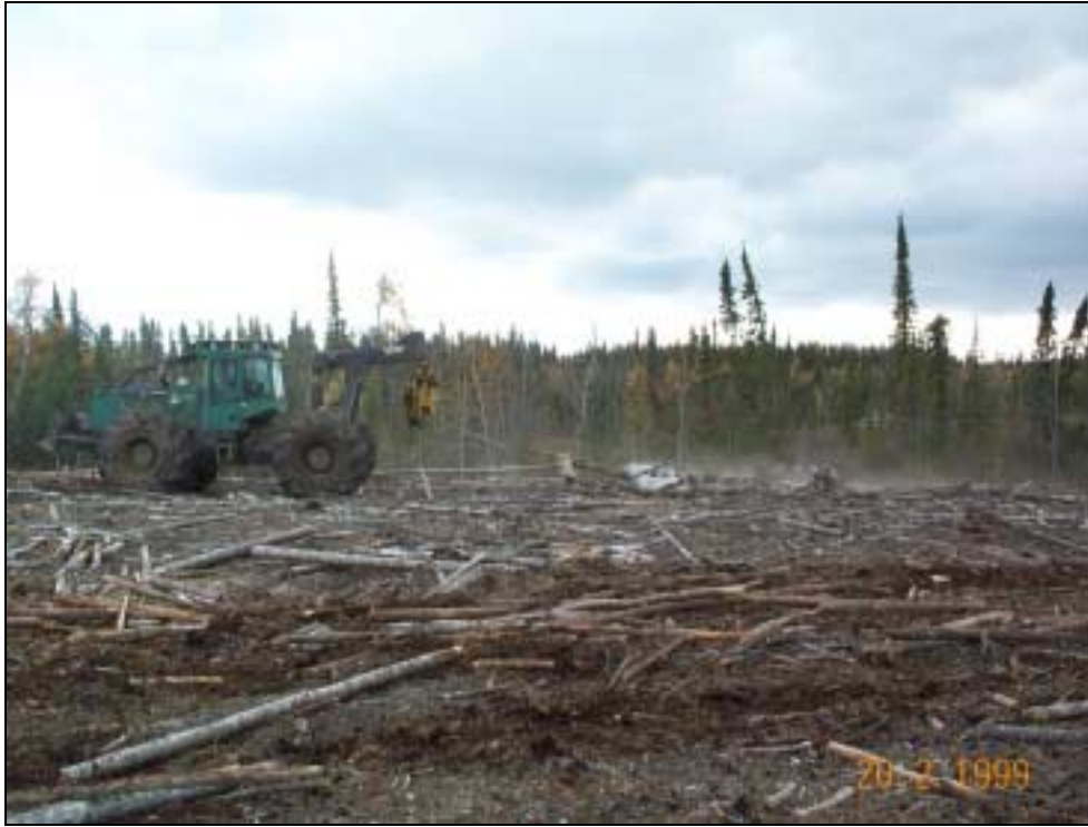
Figure 5.4 Scarification equipment – shark-fin barrels and anchor chains being pulled by a skidder.
