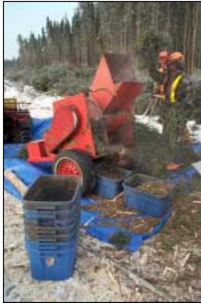
Figure 5.11 Workers feed black spruce tops into a cone combine to separate the cones from the branches.
