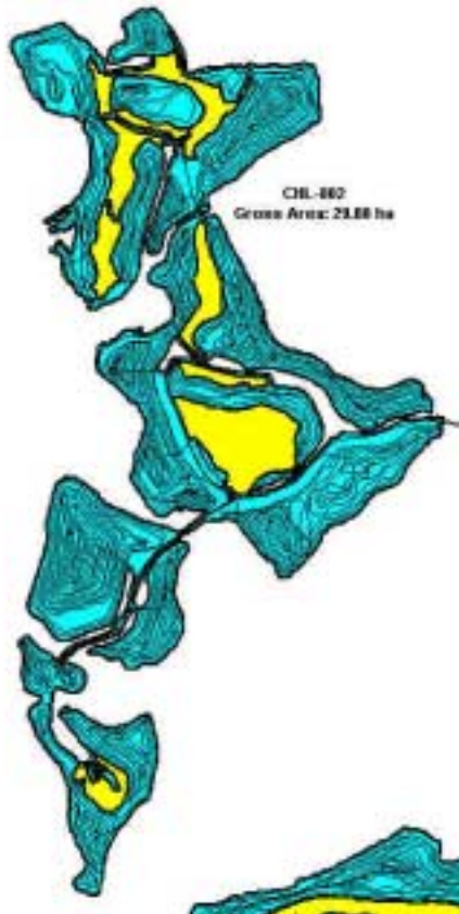
Figure 5.6 Silvitrac s map showing the exact path of the site preparation equipment. Note the leave areas (yellow residual pockets) that were not treated.
