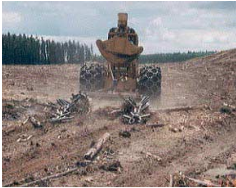
Figure 4.3 Scarification equipment – shark-fin barrels and anchor chains being pulled by a skidder.
