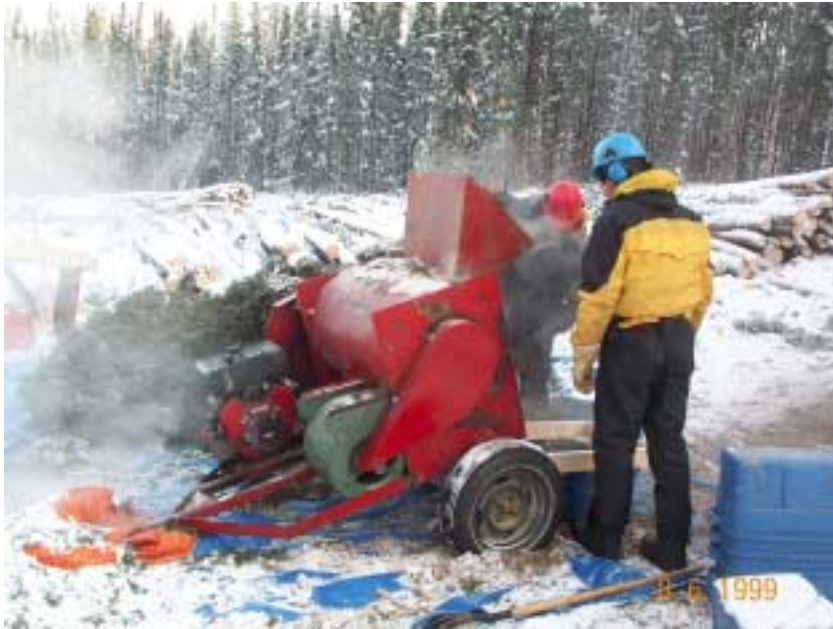
Figure 4.10 Workers feed black spruce tops into a cone combine to separate the cones from the branches.
